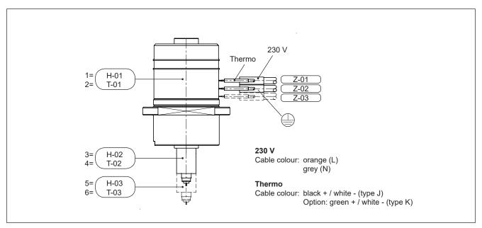
Picture 53: Wiring of HPS III-NVI single valve gate nozzles. Each control zone has a heater and a thermocouple assigned.
