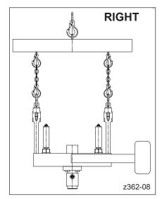
Picture 16: How to lift a load correctly using spacer bolts for attachment swivels (L2X system)
