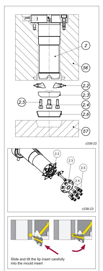
Picture 35: Installation of tip inserts
