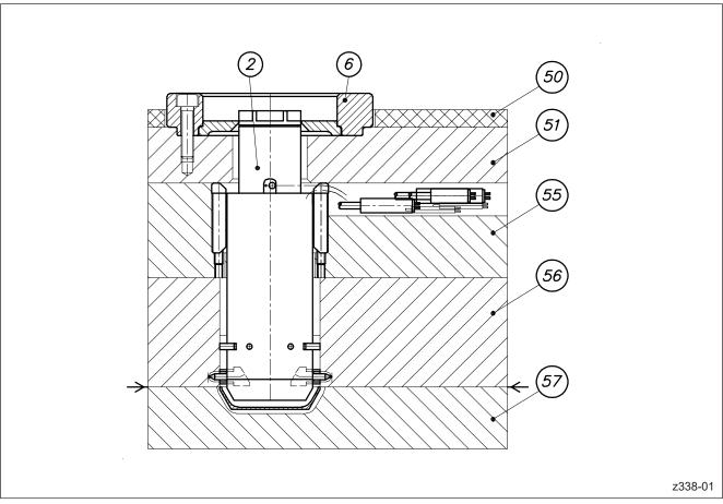
Picture 26: General layout of a system with HPS III-MHL 100/200 single tips
