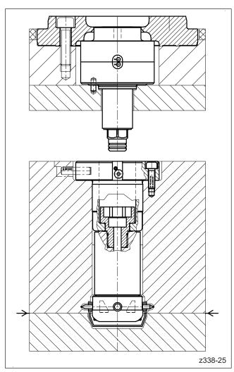
Picture 37: Installation of mould plate assemblies
