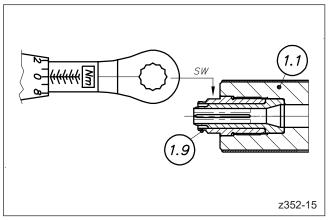
Picture 61: Tightening of nozzle tip
