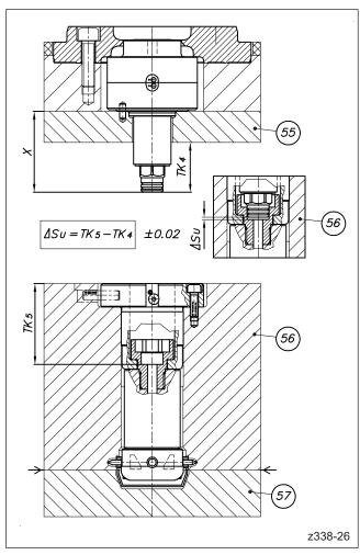
Picture 36: Check of clearance ΔS<sub>U</sub>
