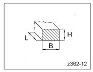
Picture 18: Dimensions of a wooden lath
