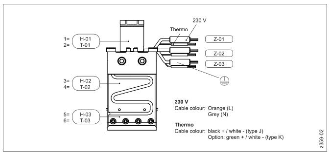
Picture 51: Wiring of HPS III-MHL single tips with three control zones. Each control zone has a heater and a thermocouple assigned.
