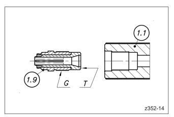
Picture 60: Installation of nozzle tip
