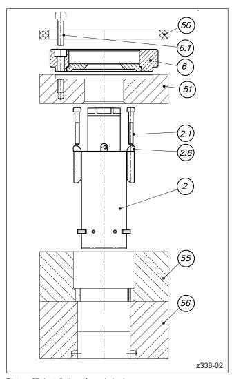
Picture 27: Installation of nozzle body
