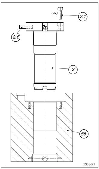
Picture 34: Installation of nozzle body
