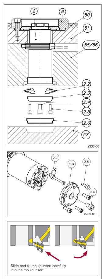
Picture 31: Installation of tip inserts
