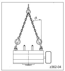
Picture 14: Lifting a load using 2 attachment points, distributed between two evenly stressed but sloping legs
