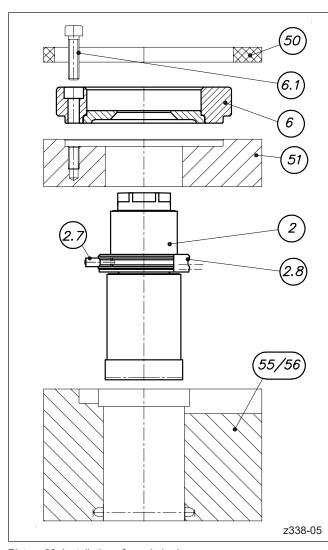
Picture 30: Installation of nozzle body
