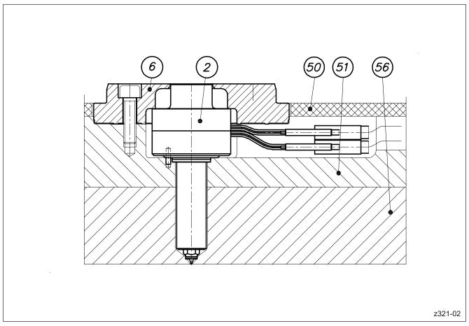
Picture 24: General layout of a system with HPS III-SXE single tips
