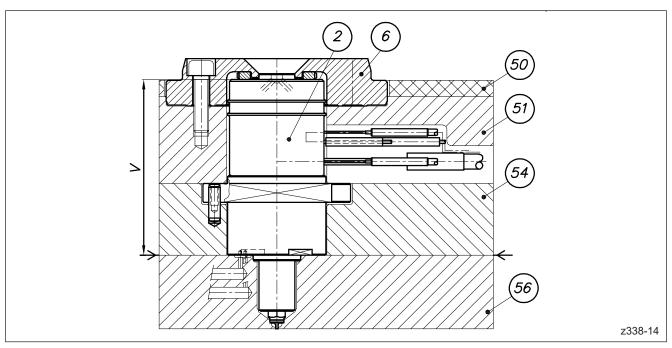
Picture 44: General layout of a system with HPS III-NVI single valve gate nozzles (Version 1 - EN306 and EN309)
