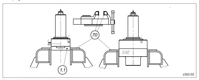
Picture 56: Clamping of a deinstalled HPS III nozzle in a vice
