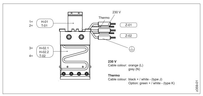
Picture 50: Wiring of HPS III-MHL single tips with two control zones. Each control zone has a heater and a thermocouple assigned.
