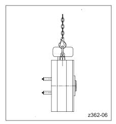
Picture 13: Lifting a load using one single attachment point
