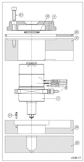
Picture 47: Installation of nozzle (Version 2)
