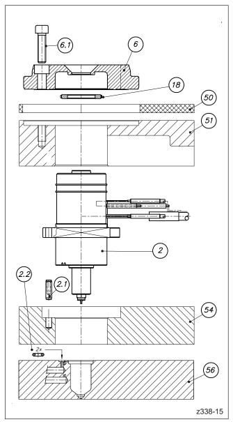
Picture 45: Installation of nozzle (Version 1)
