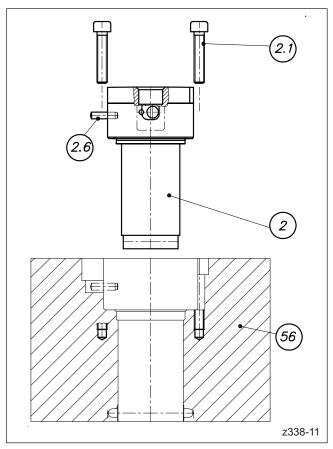
Picture 40: Installation of nozzle body
