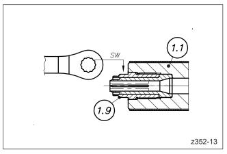
Picture 59: Unscrewing of nozzle tip
