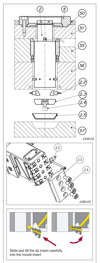
Picture 28: Installation of tip inserts
