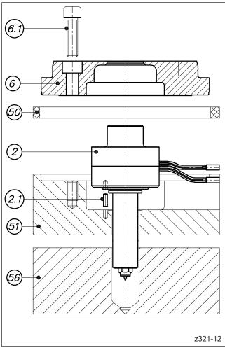
Picture 25: Installation of nozzle
