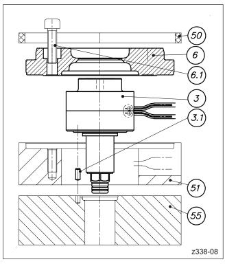
Picture 39: Installation of adapter nozzle
