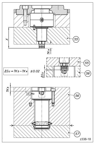
Picture 42: Check of clearance ΔS<sub>U</sub>
