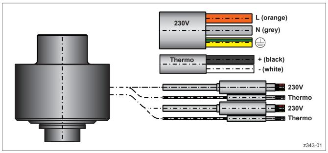
Picture 48: Cable assignments of HPS III-SXE single tips (two control zones)
