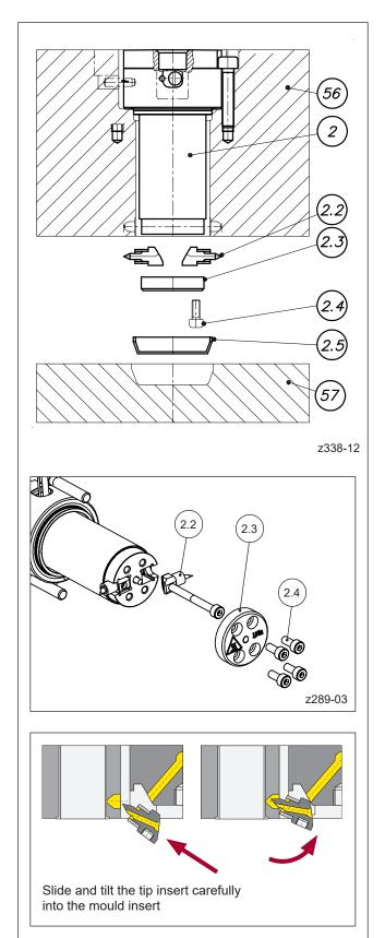
Picture 41: Installation of tip inserts
