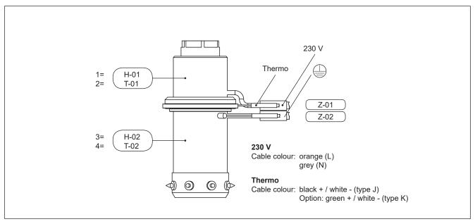
Picture 52: Wiring of HPS III-MHR single tips with two control zones. Each control zone has a heater and a thermocouple assigned.
