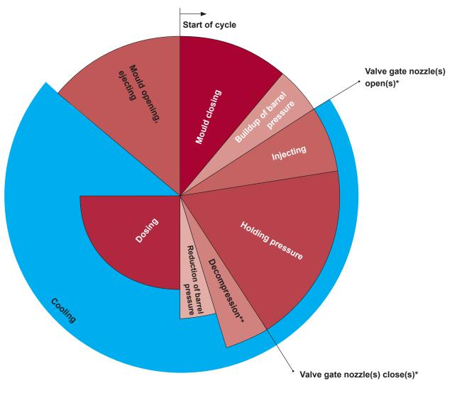
Picture 3: Injection moulding cycle
